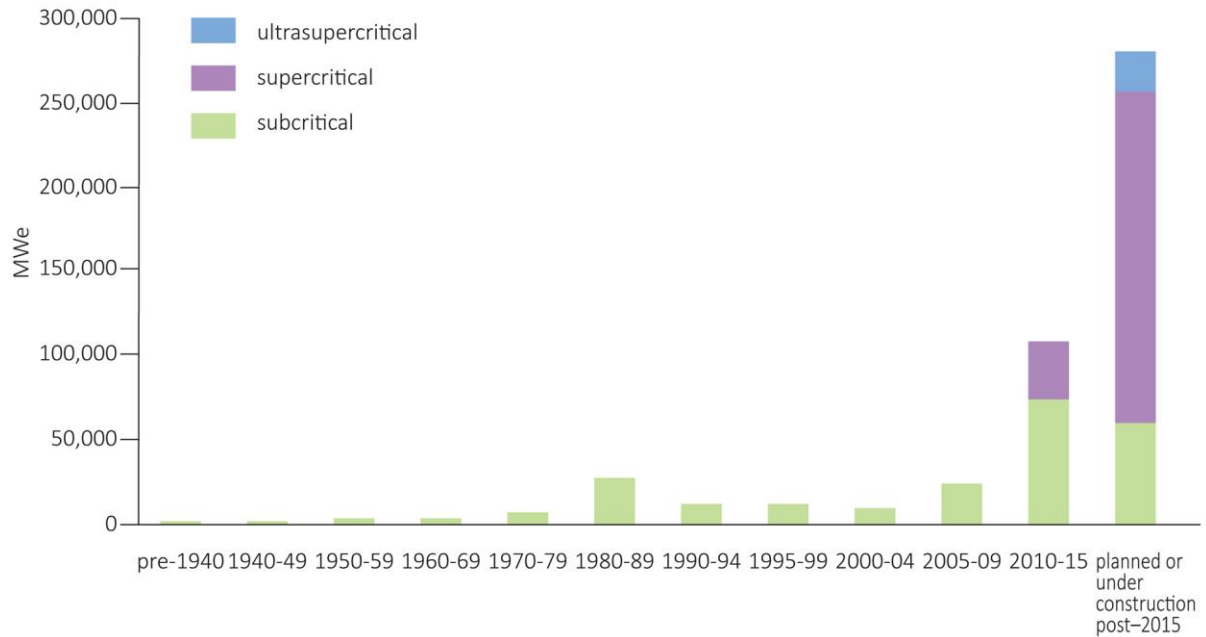
Figure 16 Indian coal-fired power plant by age and steam cycle conditions (MWe)
